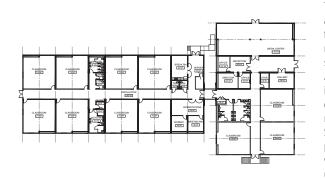
The Campus Maker ModPod provides an extensible architecture that permits fast and relatively simple addition and removal of rooms from a single large structure. For The Museum School of Avondale, the ModPod complex would include eight classrooms, a media center, male and female restrooms, and multiple ancillary rooms for faculty use. Serving an estimated twenty students per classroom, the K-3 charter school would support an enrollment base of up to 140 students in 2010-2011.
